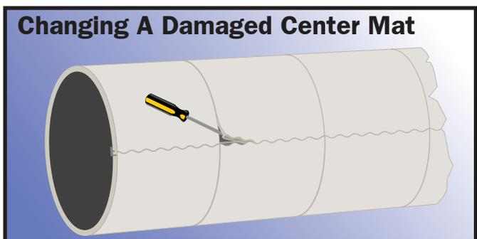
**Use a thin blade screwdriver** to raise the side of the damaged mat at the corner until it is free of the channel\*. Insert the removal tool and pull across the mat as in normal removal.
