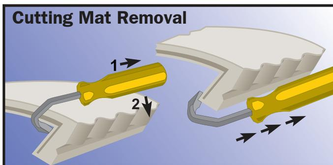
Position the removal tool's blade at the top of the slot between the surface of the cylinder and under the anvil.
